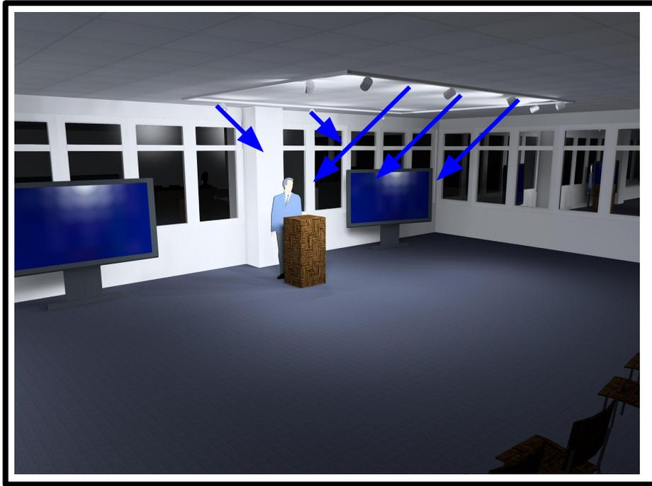
Recommended tilt angle between  $30^{\circ}$  -  $60^{\circ}$
