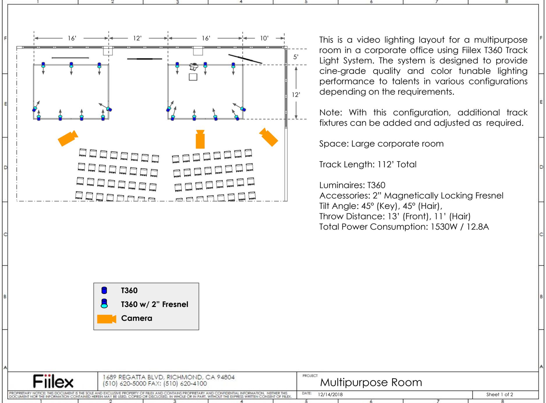
This is a video lighting layout for a multipurpose room in a corporate office using Fiilex T360 Track Light System. The system is designed to provide cine-grade quality and color tunable lighting performance to talents in various configurations depending on the requirements.
