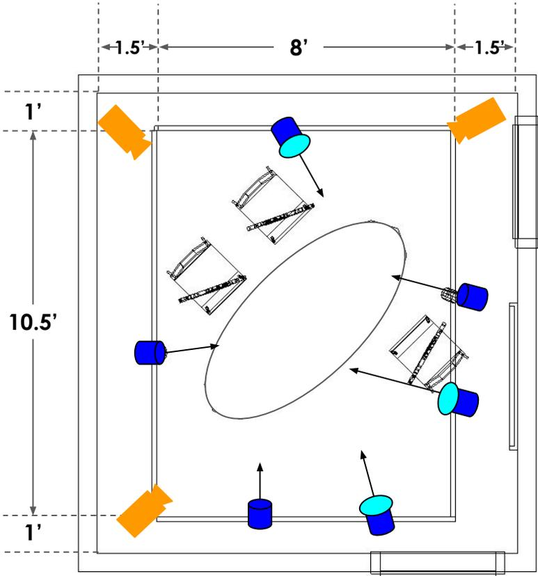
This is a video lighting layout for a small podcast studio using Fiilex T360 Track Light System. The lighting is designed for 3 talents facing each other around a table. 3 Camera are positioned inside the room, while another camera is positioned outside the glass wall.
